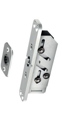
The Cable Grommet is an addition to the existing FritsJurgens top pivot range and enables wiring in the door. This top pivot contains an integrated cable grommet of  $\emptyset$ 7.5 mm. This version of the top pivot is available with every FritsJurgens system and replaces the standard delivered top pivot and ceiling plate within a complete set.
