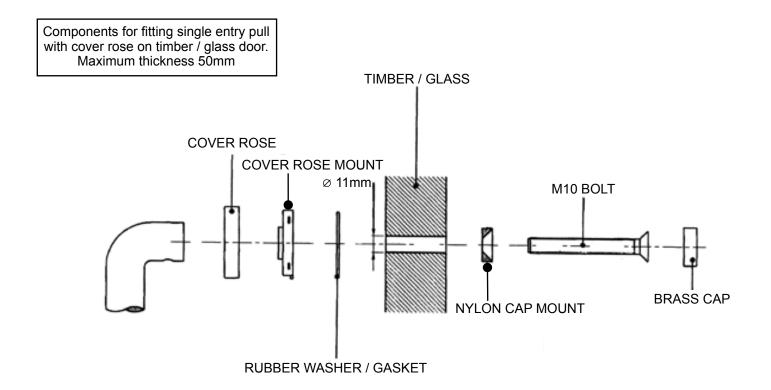
Components for fitting single entry pull on timber / glass door.
