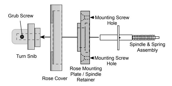
Olivari privacy turn snib used for <u>Australian</u> style locks only. Ensure lock has turn snib adapter installed in cylinder hole.
