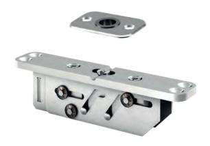
The Cable Grommet is an addition to the existing FritsJurgens top pivot range and enables wiring in the door. This top pivot contains an integrated cable grommet of  $\emptyset_{7.5}$  mm. This version of the top pivot is available with every FritsJurgens system and replaces the standard delivered top pivot and ceiling plate within a complete set.
