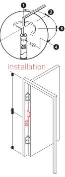
Install the spring hinge in the centre of the door between the two normal hinges.
