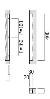
Door Suitability: timber doors 40-42mm (T2940) timber doors 36-40mm (T2941)
