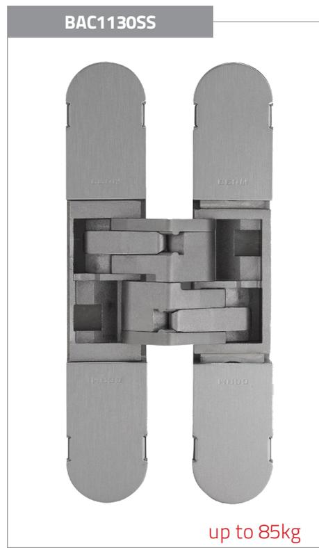
The BAC1130SS is made from AISI 304L Stainless Steel making ideally suited for internal and external environments, the BAC1130SS 3D adjustable concealed hinge is revolutionary in its design & is rated to carry upto 85kg door to 180° opening aperture.
